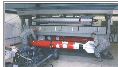
Each of the WS3 vaults at European bases can hold up to four nuclear bombs. Here crews are practicing loading B61 bombs into a vault: two B61-3/4 bombs on the top rack and two B61-12 bombs on the lower rack. Image: U.S. Air Force, obtained by Joseph Trevithick (The Drive) under FOIA. Click on image to view full size.
